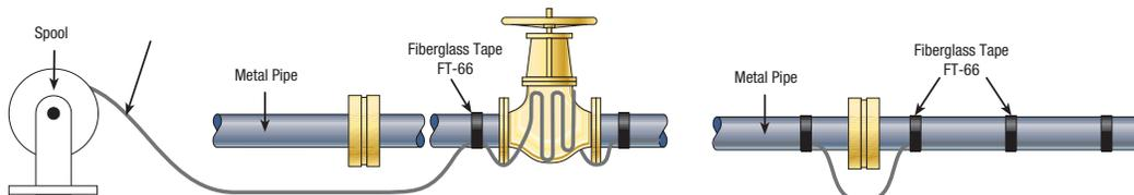
Leave a loop of cable at heat sinks such as valves, pipe supports and flange sets. Use FT-66 fiberglass tape to secure cable to pipe at 18 in. / 455 mm intervals.
